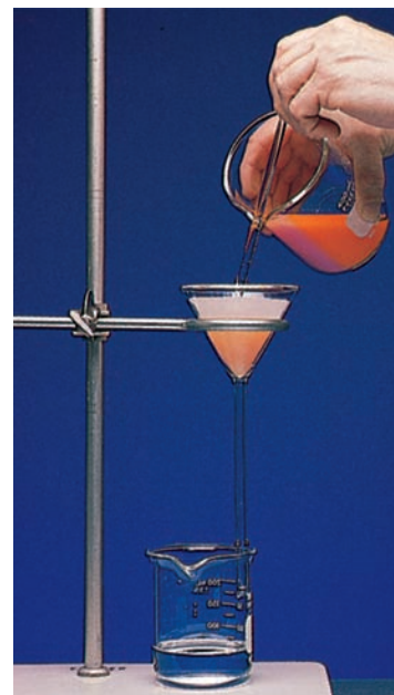
FIGURE 3-4 Filtration A heterogeneous mixture of a solid and liquid can be separated by filtration.
