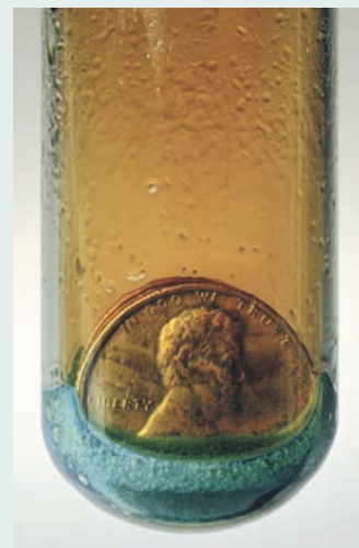
When a copper penny reacts with nitric acid, nitrogen dioxide gas (brown) is formed.
