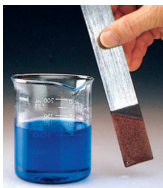
FIGURE 5-5 Single-Replacement Reaction The formation of a layer of copper on a piece of zinc is a single-replacement reaction.
