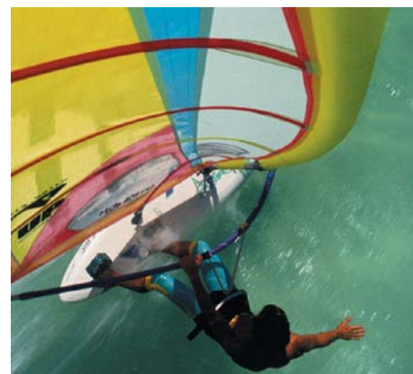
Dacron is used in these sails. It is strong, light, and does not "wet."
