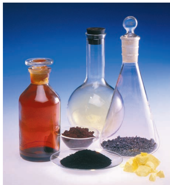
FIGURE 4-2 Nonmetals The bottle on the left contains liquid bromine and its vapor. The flask in the back contains pale-green chlorine gas. Solid iodine is in the flask on the right. Powdered red phosphorus is in the dish in the middle, and black powdered graphite (carbon) is in the watch glass in front. Lumps of yellow sulfur are shown in the front.
