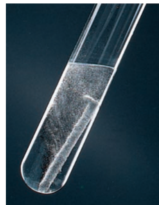
Iron is oxidized by a strong acid solution to form iron(II) ions and hydrogen gas.
