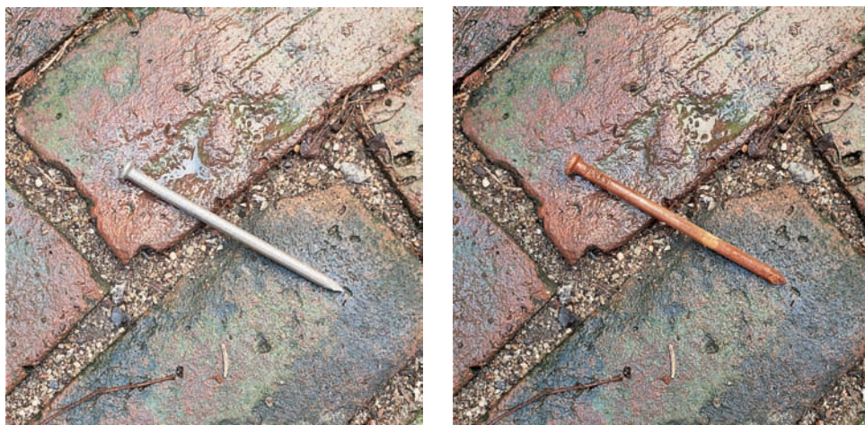
An iron nail soon forms a coating of rust when exposed to moisture and air.
