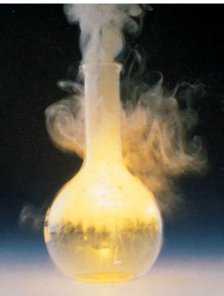
FIGURE 9-1 Reaction of Sodium with Chlorine Sodium reacts with chlorine to form sodium chloride.
