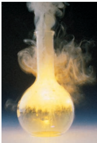
FIGURE 14-1 Formation of NaCl An active metal reacts with a poisonous gas to form ordinary table salt (NaCl).
