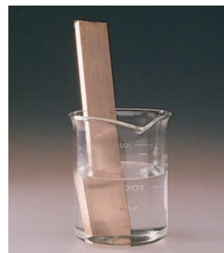
FIGURE 5-6 Copper in a Zinc Sulfate Solution When a strip of copper is immersed in a zinc ion solution, no reaction occurs.
