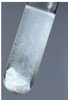
FIGURE 13-1 Zinc and Limestone in Acid Zinc (top) reacts with acid to liberate hydrogen; limestone ( \text{CaCO}_3 , bottom) reacts with acid to liberate carbon dioxide.
