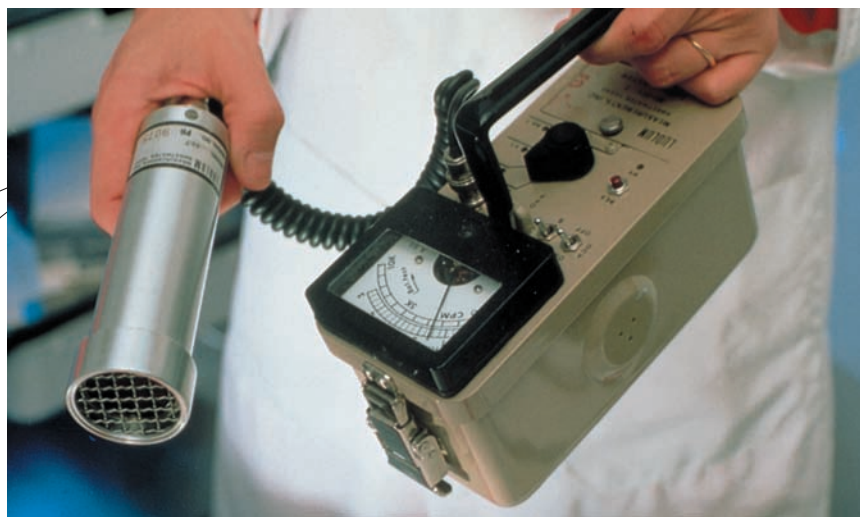
FIGURE 16-7 The Geiger Counter This device measures radiation by the ionization it causes.
