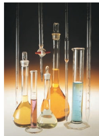
Solution volume is measured by burets, pipettes, and volumetric flasks.
