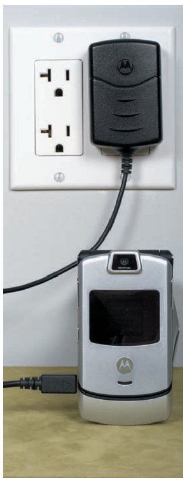
To recharge this cell phone, AC current must be converted into DC current.
