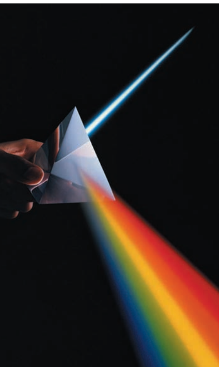
FIGURE 8-1 The Spectrum of Incandescent Light When a narrow beam of light from an ordinary lightbulb is passed through a glass prism, the white light is found to contain all the colors of the visible spectrum.
