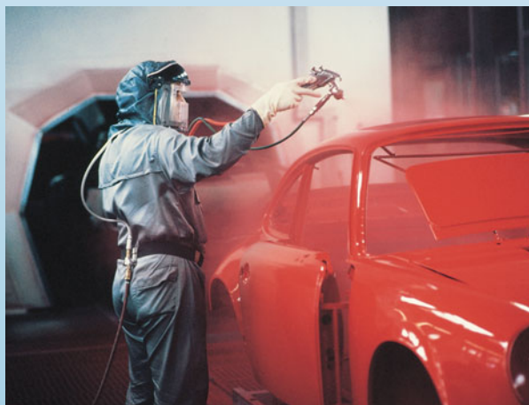
Spray painting an automobile. The worker uses a respirator to prevent inhalation of hydrocarbon solvents and other chemicals present in the paint. (Michael Rosenfeld/Tony Stone.)
