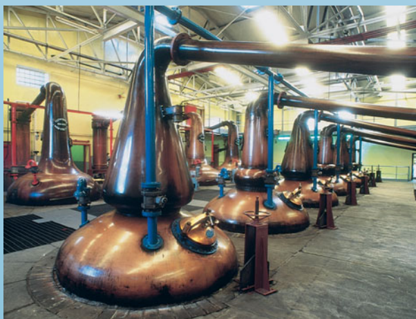
Rows of distillation stills produce whiskey at the Glenfiddich Distillery in Dufftown, Scotland. (Paul Harris/Tony Stone.)
