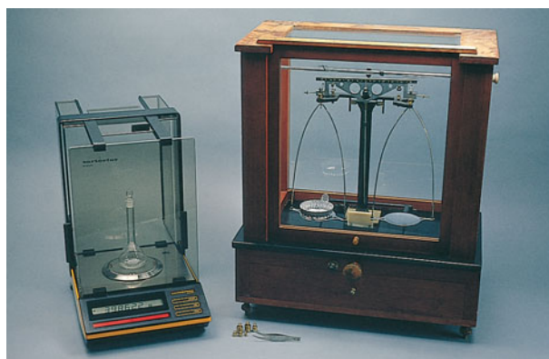
Figure 1.11 A modern automatic analytical balance ( left ) and an older laboratory beam balance ( right ). The mass of a sample on one pan of the beam balance is determined by balancing it with a known reference weight on the other pan. (Chip Clark.)
