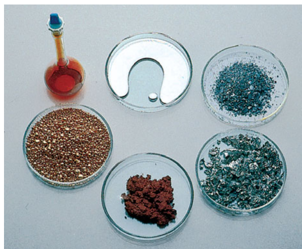
Figure 1.9 Some common elements. Clockwise from left: the red-brown liquid bromine, the silvery liquid mercury, and the solids iodine, cadmium, red phosphorus, and copper. (W. H. Freeman photograph by Ken Karp.)
