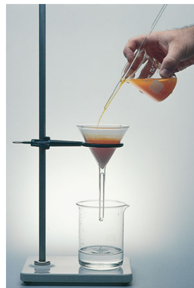
Figure 1.2 Filtration is used to separate liquids from solids. The filter paper retains the solid because the particles of the solid are too large to pass through the pores, or openings, in the paper. Micropore filters, which have pore sizes small enough to retain bacteria, are used to produce sterile water, sterile pharmaceutical preparations, and bacteria-free bottled beer. (Chip Clark.)
