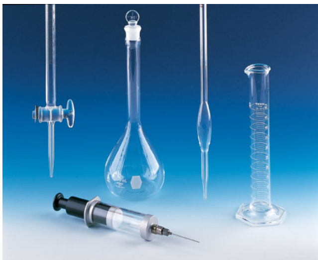
Figure 1.12 Devices for measuring liquid volumes: (back row, left to right) a buret, a volumetric flask, a pipet, and a graduated cylinder; (in front) a syringe. (Richard Megna/Fundamentals Photographs.)
