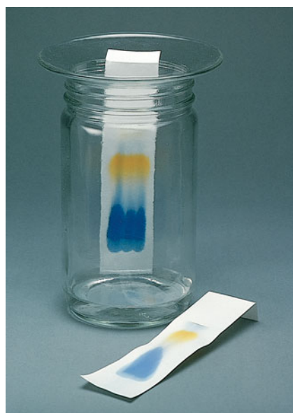
Figure 1.4 Thin-layer chromatography can separate complex mixtures and allow the identification of each compound. (Chip Clark.)
