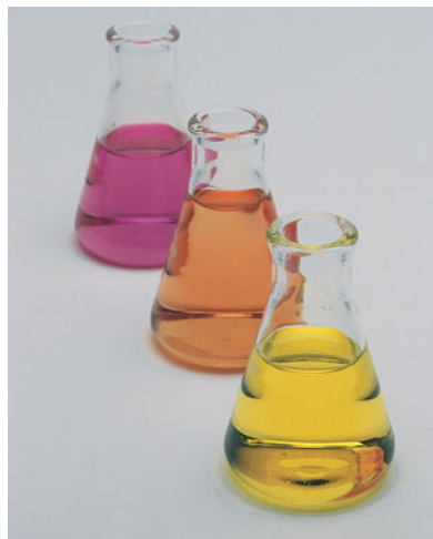
Figure 9.10 Aqueous solutions at pH 2 (red), pH 5 (orange), and pH 10 (yellow). The acid–base indicator is the dye methyl red. (Chip Clark.)
