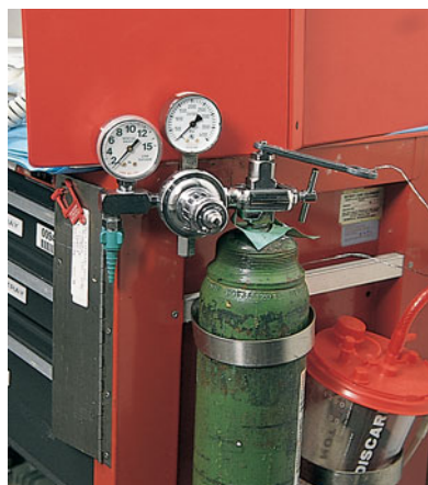
Figure 5.3 A gas-pressure gauge on a tank of oxygen used in respiratory therapy. (Mary Kate Denny/PhotoEdit.)
