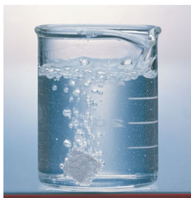
Figure 13.4 The weak acidity of an alcohol is expressed in its reaction with sodium metal to yield gaseous hydrogen ( \text{H}_2 ). (Richard Megna/Fundamental Photographs.)
