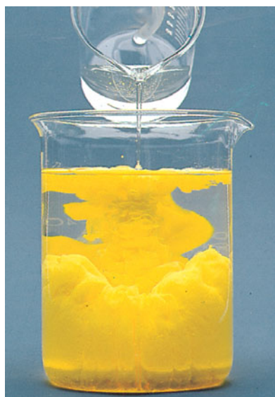
Figure 7.7 A yellow precipitate of lead(II) iodide, \text{PbI}_2 , forms immediately when colorless aqueous solutions of lead(II) nitrate, \text{Pb}(\text{NO}_3)_2 , and potassium iodide, KI, are mixed. (Chip Clark.)
