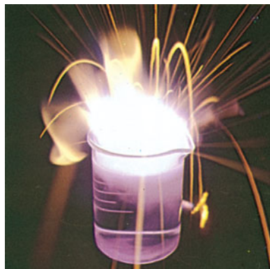
Figure 2.4 The violent reaction of the alkali metal potassium with water. The products of the reaction are hydrogen gas and potassium hydroxide, as well as lots of heat. The flames are a result of the hydrogen reacting with oxygen from the air. The sparks are pieces of the molten potassium driven into the air by the force of the explosion. (Alexander Boden.)
