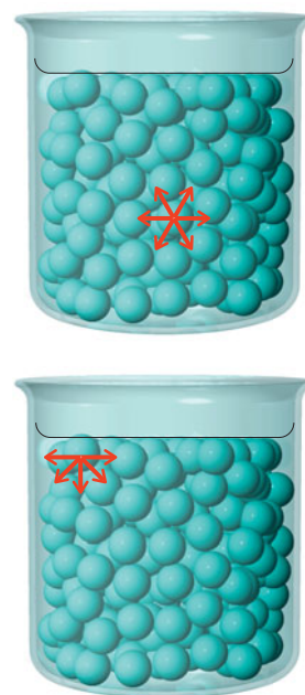
Figure 6.6 Molecules in a liquid are attracted in all directions, but molecules at the surface are attracted only in an inward direction. The inward pull results in surface tension.
