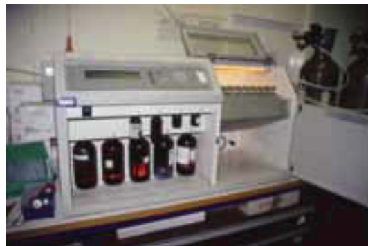
Figure 17.3 Automated instrument for the extraction of DNA from blood samples of 5–20 ml volumes
