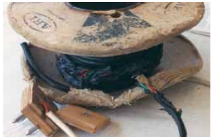
Frayed electrical cable and homemade plug discovered at a work site
