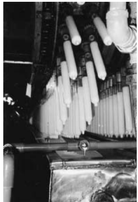
Figure 2.3 Latex condoms emerging from a dripping tank in the factory
