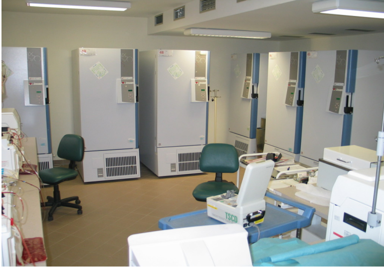
Fig. 3. Mechanical freezers for deep freezing (-65°C - -80°C)
