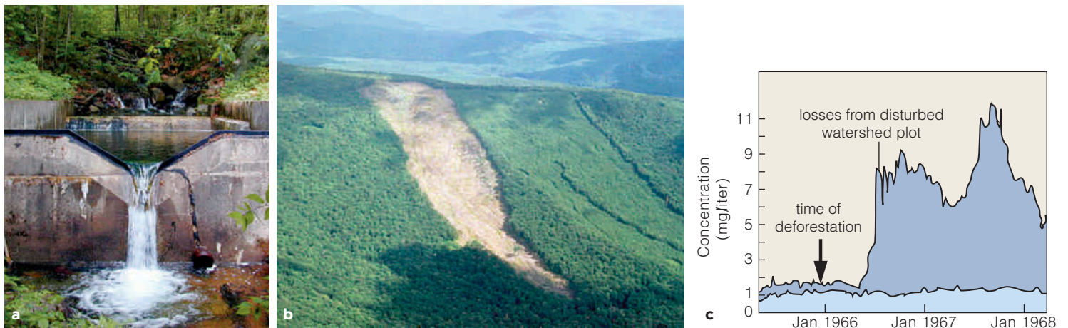
Figure 47.12 Hubbard Brook experimental watershed. (a) Runoff in this watershed is collected by concrete basins for easy monitoring. (b) This plot of land was stripped of all vegetation as an experiment. (c) After experimental deforestation, calcium levels in runoff increased sixfold ( medium blue ). A control plot in the same watershed showed no similar increase during this time ( light blue ).
