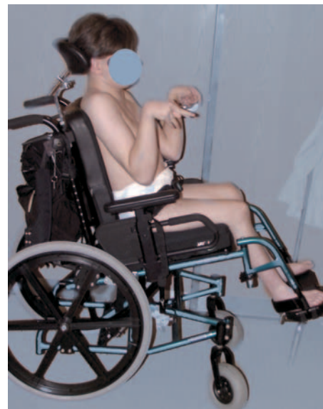
Figure 6.32. The tilt-in-space frame allows the child to lie back with loosening of the seating positioning. The tilt-in-space frame tilts both the seat and back at the same time compared with a reclining wheelchair, in which the back folds down but the seat stays in place.
