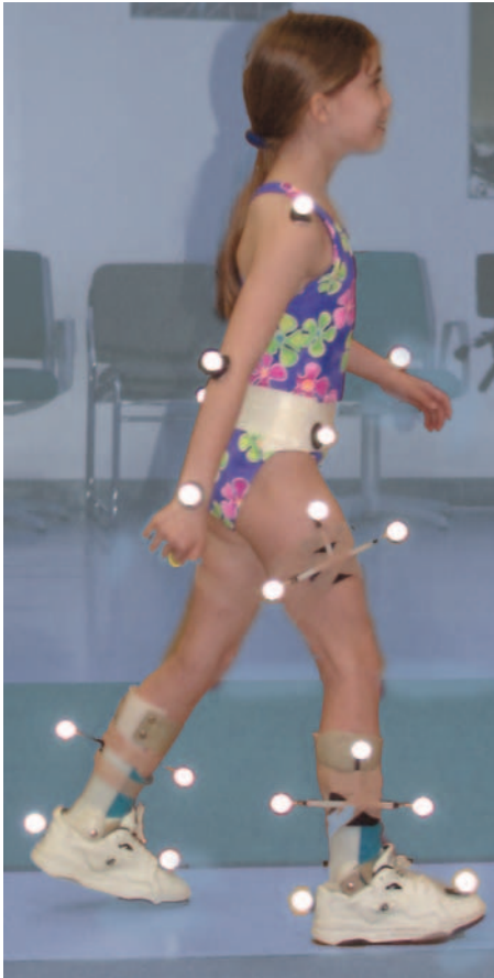
Figure 7.11. The most common gait measurement system requires that the individual being measured is instrumented with retro-reflective markers that are imaged by multiple video cameras. The markers define specific anatomic body points, which the computer program uses to calculate joint motion.
