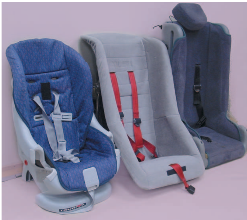
Figure 6.46. The car seats for children with disabilities are very similar to those sold for children without disabilities, except the special needs car seats are designed for much larger children.
