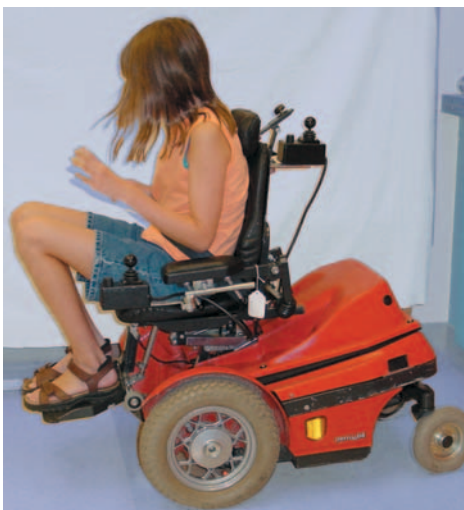
Figure 6.31. The deluxe power wheel base (A) allows power floor sitting (B), standing, seat raising, reclining, tilt-in-space, and foot elevation. These systems are expensive and often require a high level of maintenance.
