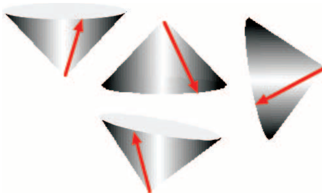
Figure 5.3 Depiction of four spinning nuclei. Spinning nuclei simultaneously spin and precess at a Lamor frequency , \nu_L , therefore angular momentum vectors (red arrows) map out precessional cones. In the absence of any external magnetic field, vectors align relative to arbitrary z -axes. According to quantum mechanical rules, magnitude of angular momentum J is determined by spin quantum number I and a spinning nucleus can exist in any one of 2I + 1 spin states.
