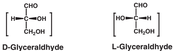
Figure 1.35 D- and L-glyceraldehyde to illustrate principles of the Fischer Projection . The D and L absolute configuration convention for all sugars refers to the stereochemistry of the bracketed terminal carbons whose configuration is compared with the two enantiomers of glyceraldehyde.
