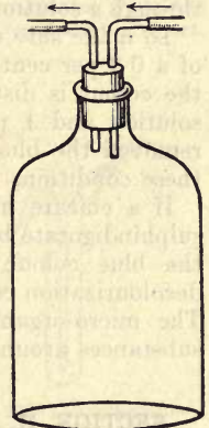
FIG. 77.—Wash-bottle fitted up for use with a water pump to prevent backflow of water into the culture medium.
